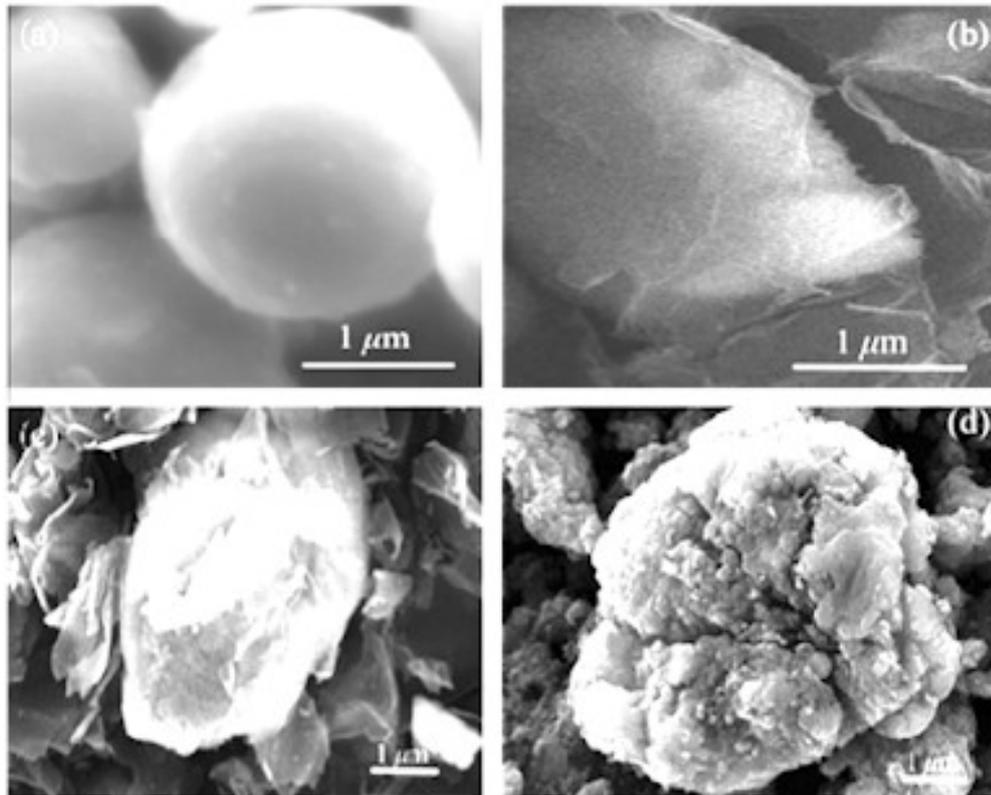
*Fig. 11. Table C) F-CIP coated graphene oxide compound (Xu, Y .; Luo, J .; Yao, W .; Xu, J .; Li, T. 2015)*
