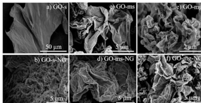
Fig. 10. Corrugation morphology of graphene oxide samples (Quan, L. ; Qin, FX; Estevez, D. ; Lu, W. ; Wang, H. ; Peng, HX 2019)
