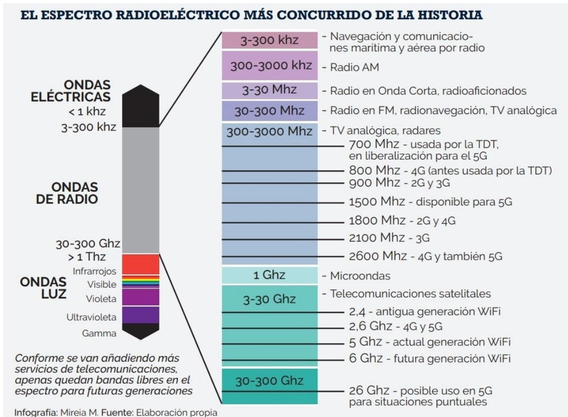
Fig. 1. Radio spectrum scheme
