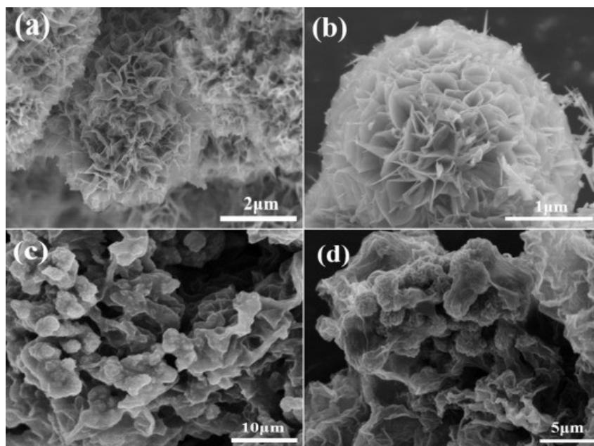
Fig. 5. Flower-shaped reduced graphene oxide nanosheets (Hu, J. ; Shen, Y. ; Xu, L. ; Liu, Y. 2020)
