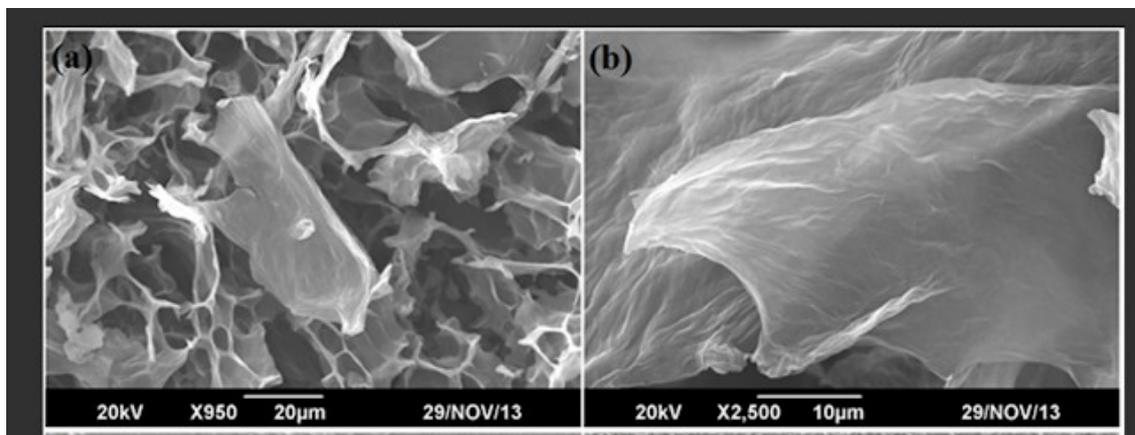
Fig. 3. Sample nanomaterial of NiFe<sub>2</sub>O<sub>4</sub>-rGO
