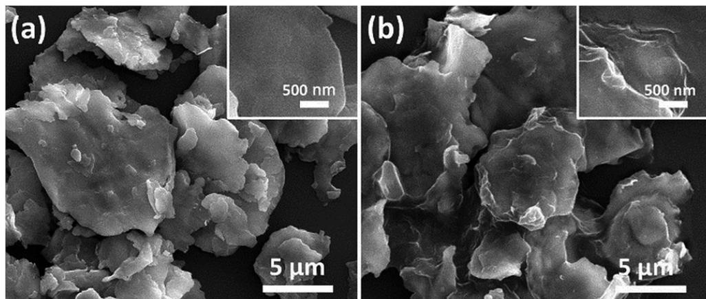
*Fig. 7. RGO-coated scaly carbonyl iron (He, L .; Zhao, Y .; Xing, L .; Liu, P .; Wang, Z .; Zhang, Y .; Du, Y. 2018)*
